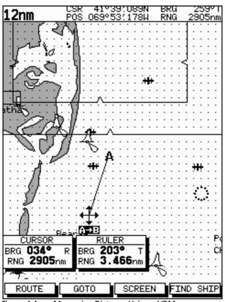
Figure 4-1: Measuring Distance Using a VRM
